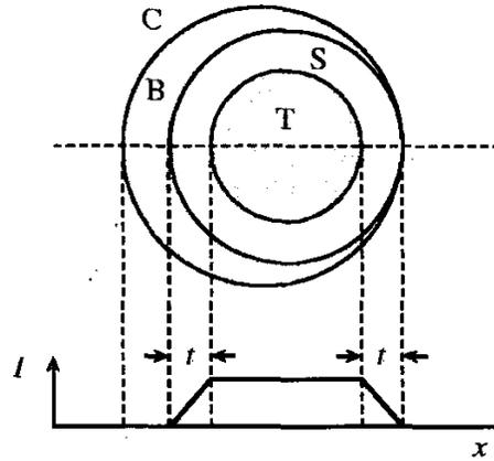
Figure 4. Circular object with a broad slope edge  $S$  of width  $t$ , lying just within a circular window  $C$ . The two shaded regions  $T$  (top of object) and  $B$  (background) have equal area. Shown below is the side view along the middle of the window which represents the intensity  $I$  on passing right through the circular object.
