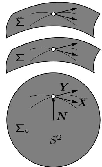
**Theorem.** A shell membrane  $\Sigma$  with vanishing ‘shear’ stress and constant purely normal loading is in equilibrium if and only if there exists a Combescure transform  $\tilde{\Sigma}$  such that the **orthogonality condition**
