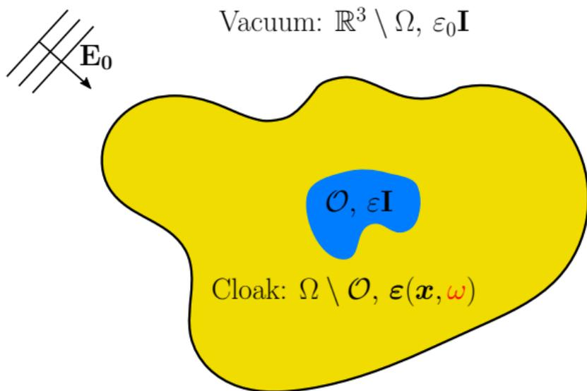
**Issue:** is it possible to construct a **passive cloak** that will cloak a dielectric inclusion  $\mathcal{O}$  over a **whole frequency band**:  $[\omega_-, \omega_+]$ ?
