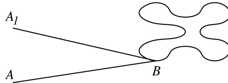
How it works:  $\text{Area} \approx |AB||AA_1|$ , the more accurate, the larger  $|AB|$  is (a power series expansion in  $1/\ell$ ).
