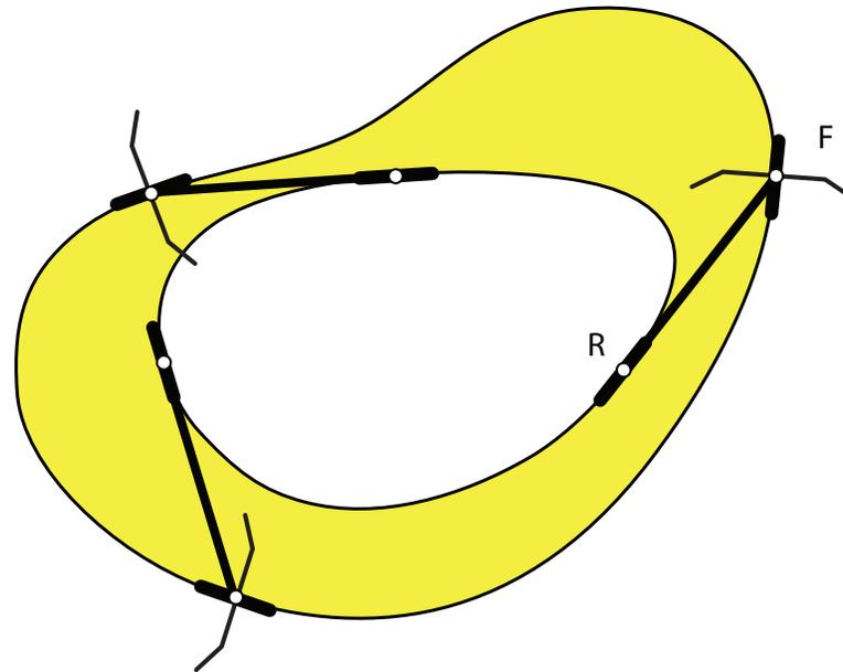
Segment  $RF$  moves so that the trajectory of  $R$  is tangent to the segment. *Notation:*  $\gamma$  is the rear track,  $\Gamma$  is the front track. When the steering angle is  $90^\circ$ ,  $\gamma$  has a cusp. One can do it in  $\mathbf{R}^n$ , and on a Riemannian manifold. (animation)
