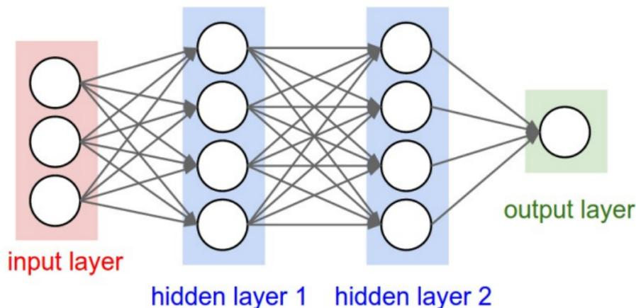
Figure: A regular 3-layer Fully Connected Neural Network.<sup>1</sup>
