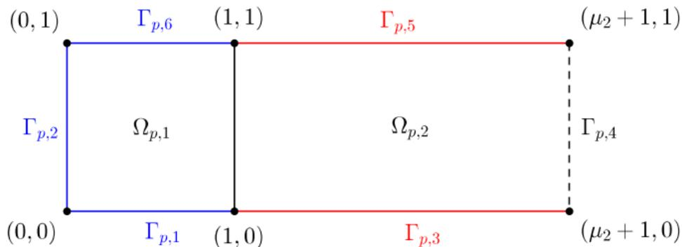
$$\begin{cases} -\frac{1}{\mu_1} \Delta u(\mu) + 4y(1-y) \partial_x u(\mu) = 0 & \text{in } \Omega_p(\mu) \\ u(\mu) = 0 & \text{on } \Gamma_{p,1}(\mu) \cup \Gamma_{p,2}(\mu) \cup \Gamma_{p,6}(\mu) \\ u(\mu) = 1 & \text{on } \Gamma_{p,3}(\mu) \cup \Gamma_{p,5}(\mu) \\ \frac{1}{\mu_1} \frac{\partial u}{\partial n} = 0 & \text{on } \Gamma_{p,4}(\mu). \end{cases}$$
