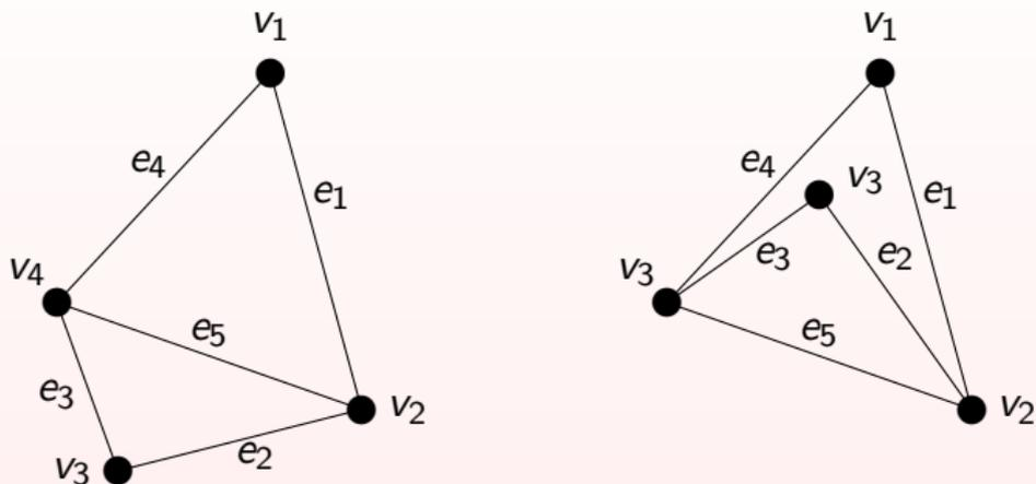
Figure : A rigid 2-dimensional framework which is not globally rigid. All edges in both frameworks have the same length, but the distance from  $v_1$  to  $v_3$  is different.
