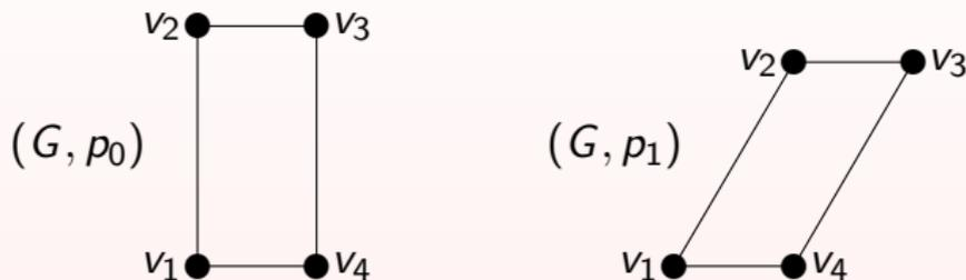
**Figure :** A 2-dimensional example. The framework  $(G, p_1)$  can be obtained from  $(G, p_0)$  by a continuous motion which preserves all edge lengths, but changes the distance between  $v_1$  and  $v_3$ . Thus  $(G, p_0)$  is not rigid.
