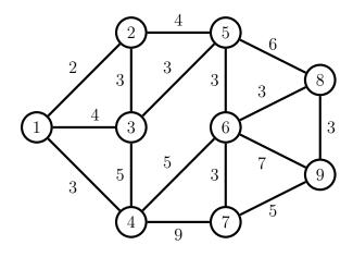
The numbers on the arcs denote distances between nodes. Apply Dijkstra's algorithm to find the shortest distance from node 1 to node 9. Identify the corresponding shortest paths from node 1 to node 9.
