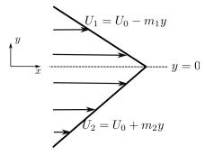
The basic velocity vector does not have a vertical component (in the y direction) and its horizontal component (in the x direction) is given as
