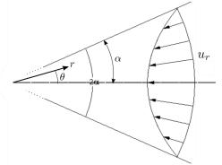
We assume that the flow is 2D ( $u_z = 0$  and  $\partial/\partial z = 0$ ), and satisfies the incompressible, steady state Navier Stokes equations in polar coordinates. For the velocity, we assume the following form
