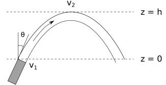
The flow leaves the hose at speed  $v_1$  and is travelling horizontally at speed  $v_2$  when the flow reaches its highest point. The only force acting on the flow is gravity so that  $\mathbf{f} = -g\mathbf{e}_z$ . Assuming that pressure is constant within the flow use Bernoulli's function to find *h* in terms of *g*,  $v_1$  and  $\theta$ .
