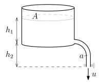
We will model the beer as an incompressible, inviscid fluid, flowing steadily under gravity.
