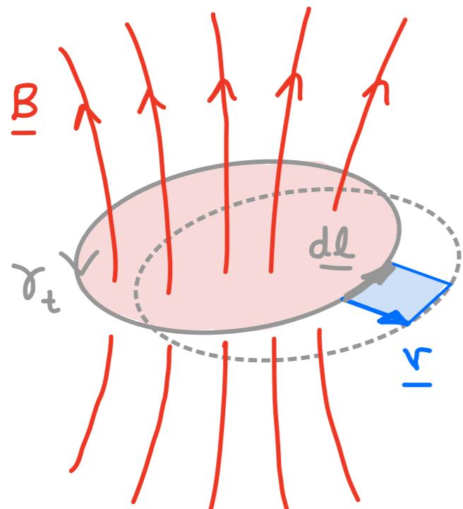
flux through a material curve (moving with fluid)
