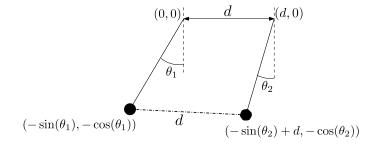
The velocity of the left hand mass is simply  $((-\cos(\theta_1)\dot{\theta})_1^2 + (\sin(\theta_1)\dot{\theta}_1)^2) = \dot{\theta}_1^2$ . We get a similar result for the right hand mass so the total kinetic energy T is
