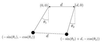
The velocity of the left hand mass is simply  $((-\cos(\theta_1)\dot{\theta})_1^2 + (\sin(\theta_1)\dot{\theta}_1)^2) = \dot{\theta}_1^2$ . We get a similar result for the right hand mass so the total kinetic energy T is
