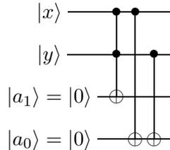
In this case the order of the gates doesn't matter. The CCNOT gate sets  $a_1 = 1$  if  $x = y = 1$  while the two CNOT gates set  $a_0 = 1$  if precisely one of  $x = 1$  or  $y = 1$ .
